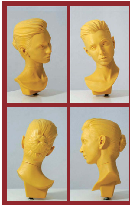
"Jesse" by sculptor Frank Benson is a bust produced first as a mold-master on an Envisiontec Perfactory Xede system at Morpheus Prototypes, then cast in bronze. Images courtesy Morpheus Prototypes.
